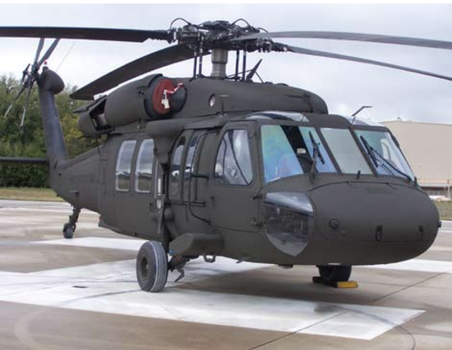
Blackhawk helicopter testbed for Type II waterborne CARC technology at Fort Hood, TX. All helicopters on the base are now repainted using waterborne CARC.
