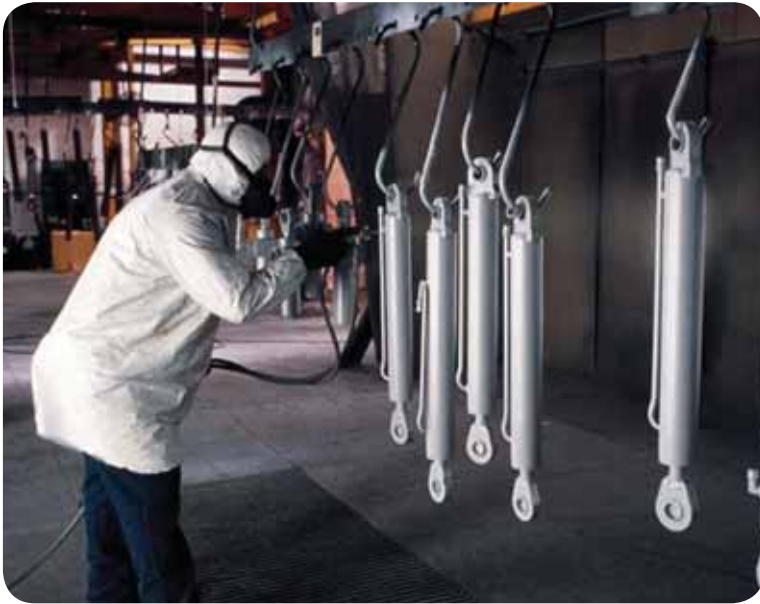
The use of polyurethane coatings has been increasing in the manufacture of farm equipment.
